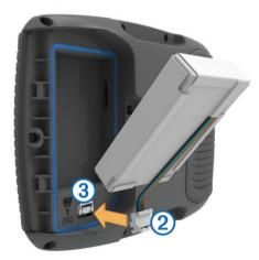
6 Close the battery cover and secure the battery cover D-ring.
