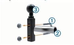
2 Tighten the nuts to secure the base.
